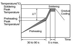
[Allowable Flow Soldering Temperature and Time]
