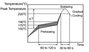
[Allowable Reflow Soldering Temperature and Time]
